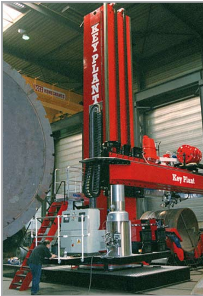
10m x 8m Column & Boom for the manufacture of pressure vessels
