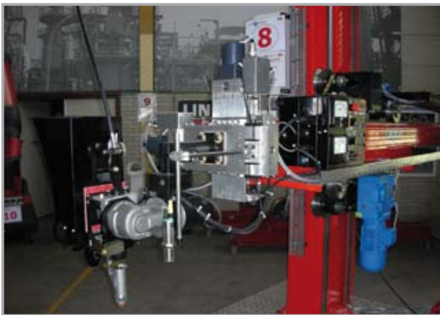
Height Sensing System for sub arc
