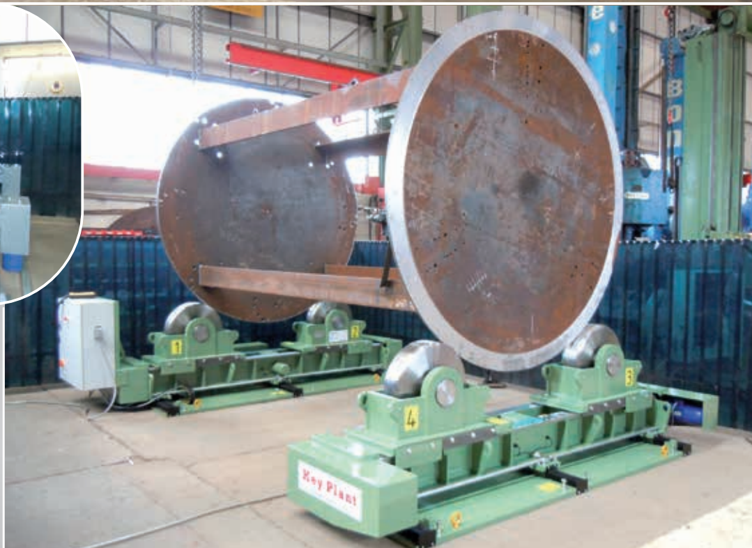
1000 Ton Fit Up Rotators designed for the alignment of heavy wall tubes & components. Each wheel carriage has independent motorised adjustment.
