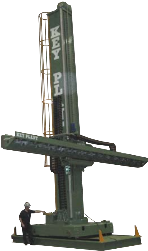
11m x 11m Extra Heavy Duty Column & Boom Manipulator
