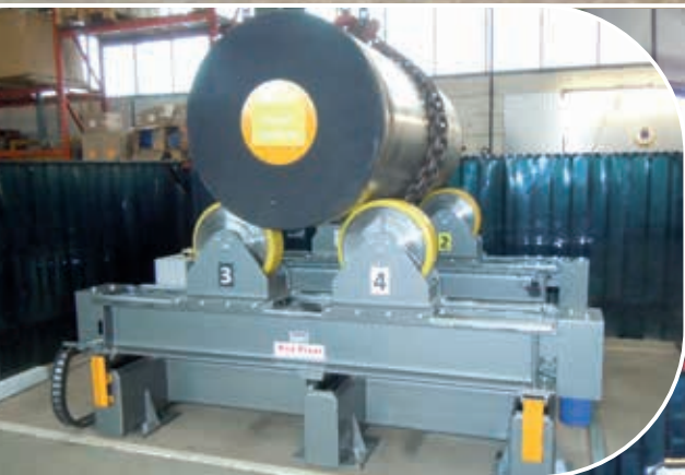
100 Ton Fit Up Rotators with motorised travel for longitudinal and horizontal cross slide travel.
