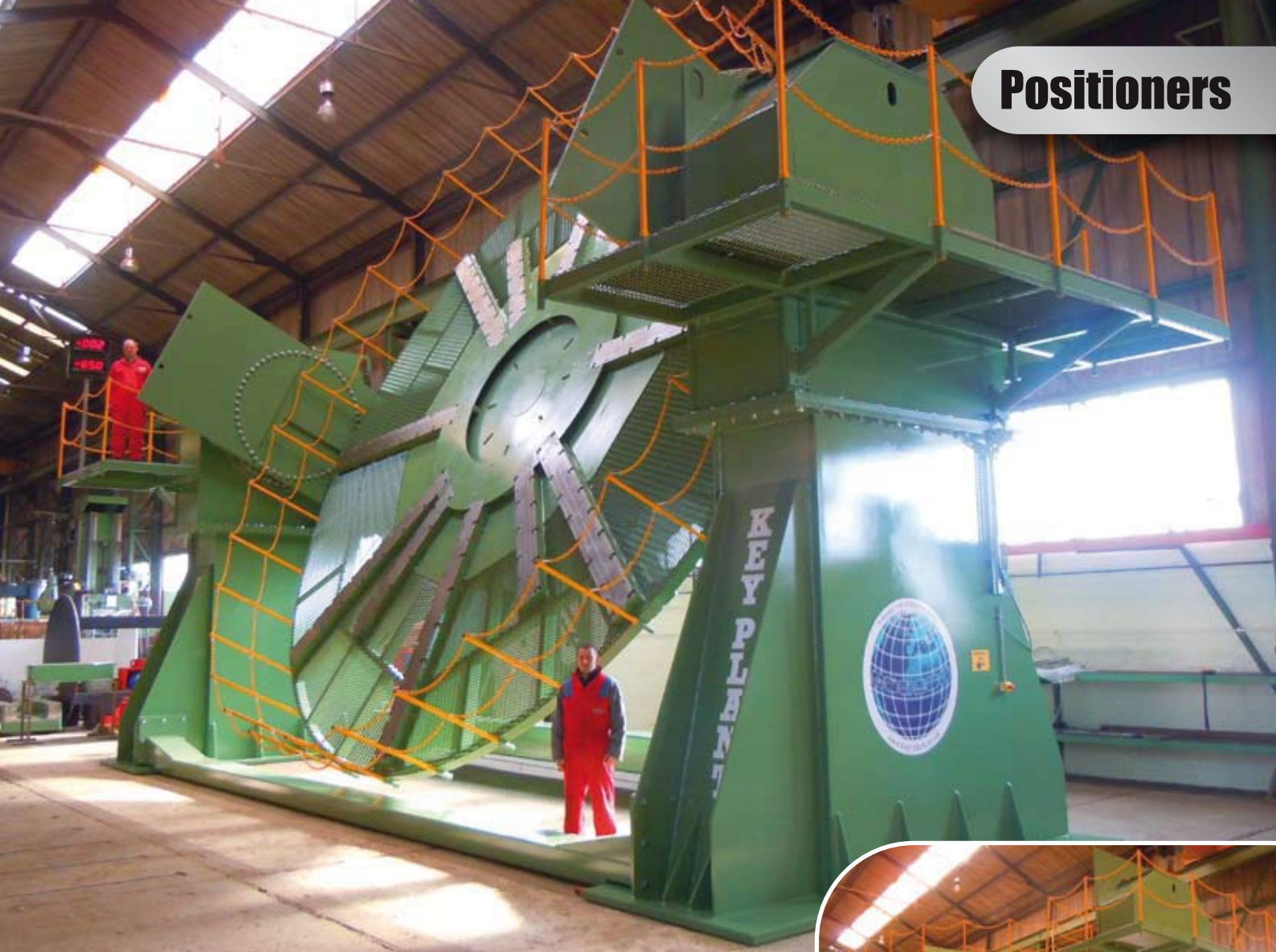
500 Ton Cradle Type Positioner with 9,200mm diameter table
