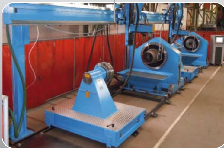
Headstocks being built at Key Plant's factory in Leek, UK.
