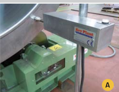
500 Ton Conv Rotators with Twin Anti-Drift System
