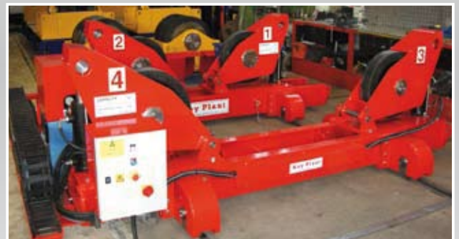
Traversing Elevating Rotators for the manufacturing of thick walled pipes and parts
