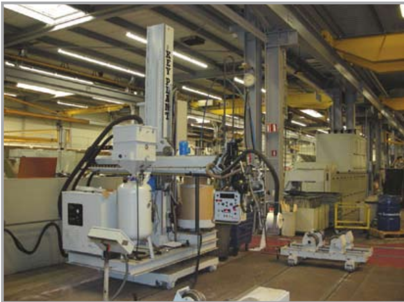
Mid Duty Welding System for the manufacture of hydraulic cylinders
