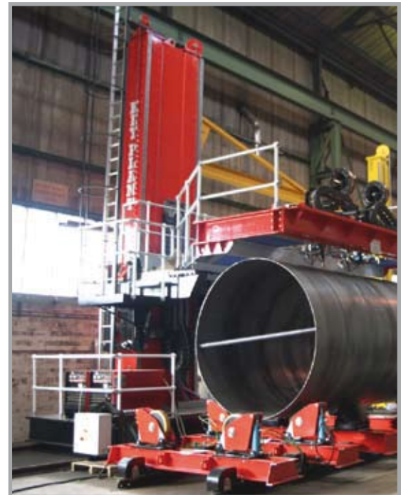
8m Platform Twin Head Welder for the manufacture of double & single skinned storage tanks
