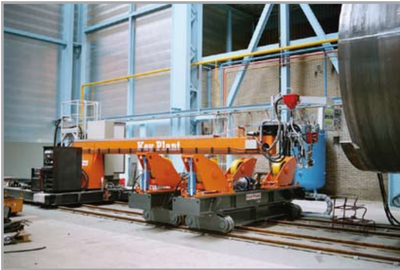
Internal Boom Welding Station for fit up with Tandem Welding with Elevating Idlers
