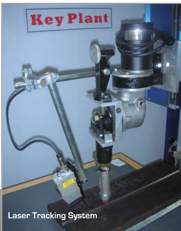
Height Sensing System for sub arc
