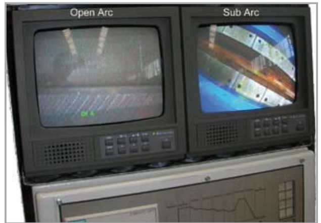
Vision Systems for sub merged arc and open arc
