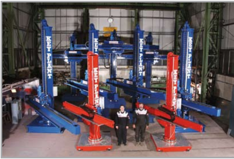
4m x 4m and 5m x 5m Column & Boom for export for the cladding of offshore valves
