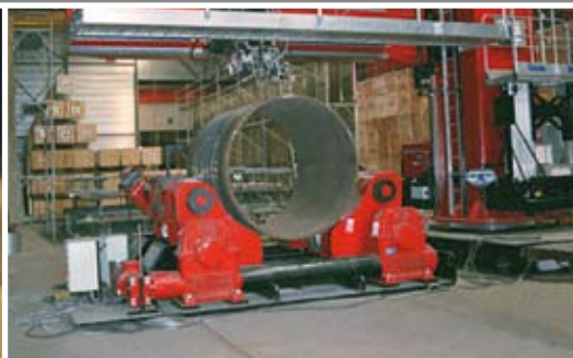
400 Ton SAR Rotators with Twin Anti-Drift system
