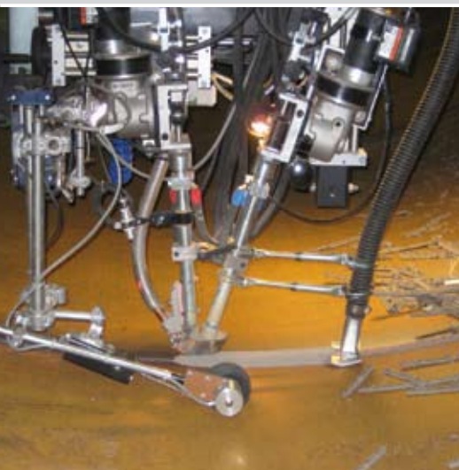
Tandem Welding with 4 welding wires
