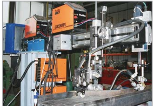
Side Beam Installation with Tracking System for the manufacture of truck bodies
