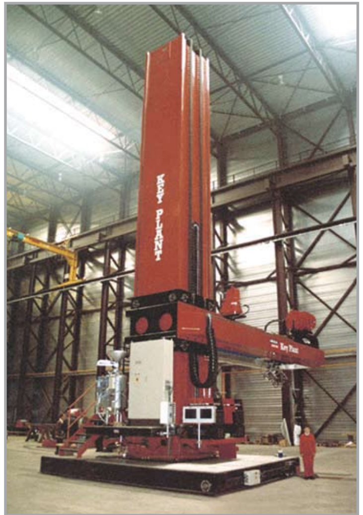
15.5m x 10m Traversing Column & Boom for manufacturing of nuclear vessels, Europe's largest Column & Boom
