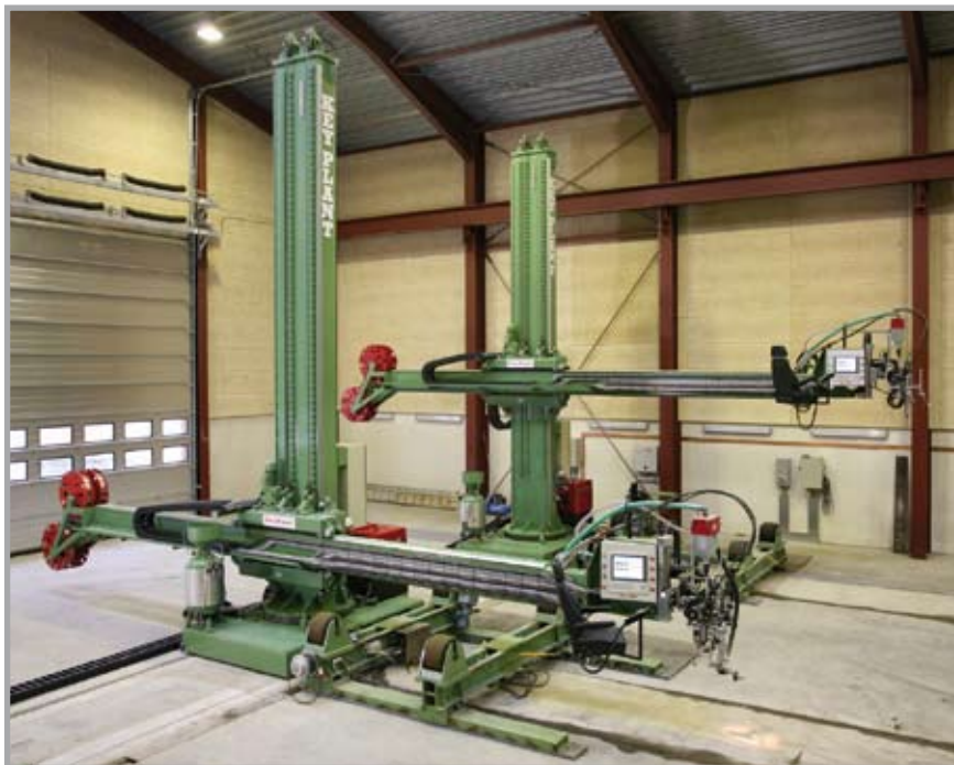
9m x 9m Traversing Column & Boom for wind tower production
